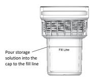
b. Carefully screw the cap with storage solution onto the logger.
