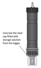
If you removed the clear storage cap, screw the closure cap onto the logger.
