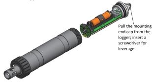
4. Remove the battery strap. Insert a flat-head screwdriver into the hole on the strap to lift it off the battery.
