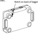
Insert the black base of the attachment into the notch so that the base clips onto the corner of the logger as shown below.
