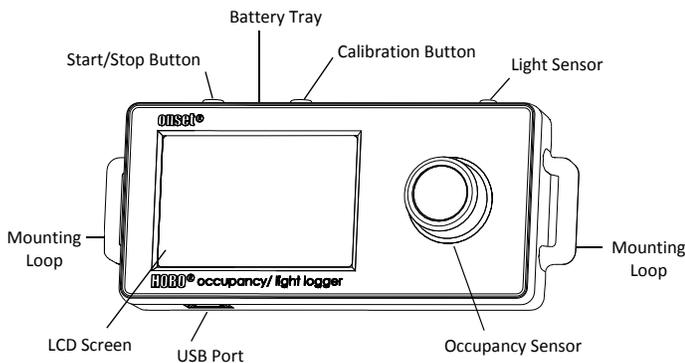
**Start/Stop Button:** Press this button for 3 seconds to start or stop logging data. This requires configuring the logger in HOBOWare with a push button start or stop (see *Setting up the Logger*). You can also press this button for 1 second to record
