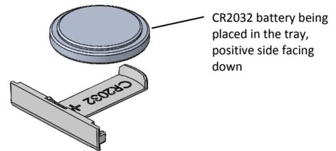
4. With the LCD screen still facing up, slide the tray back into the logger. The LCD should display “HOBO” briefly after correctly installing the battery.
