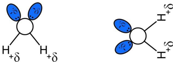
Figure 4.2. A water molecule in the liquid phase reorienting i.e. rotational dipole moment.
