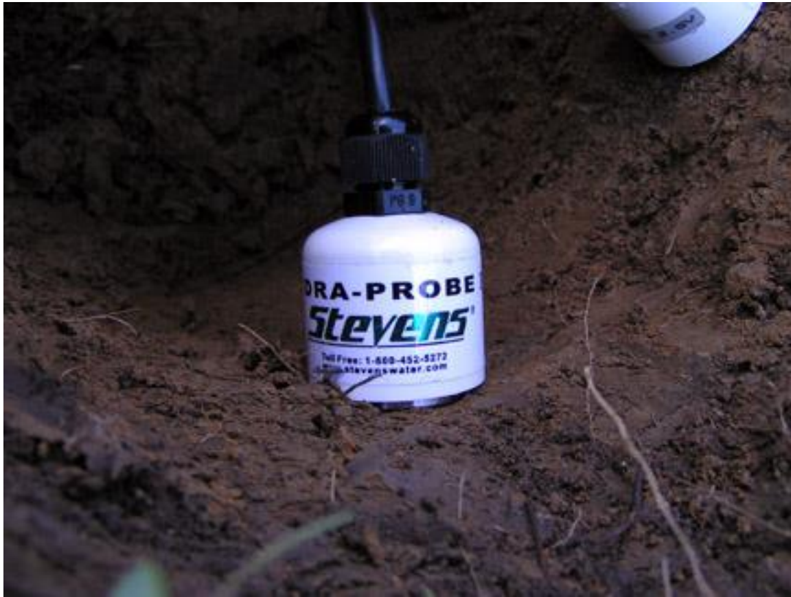
Figure 3.5 Hydra Probe Installed in undisturbed soil.
